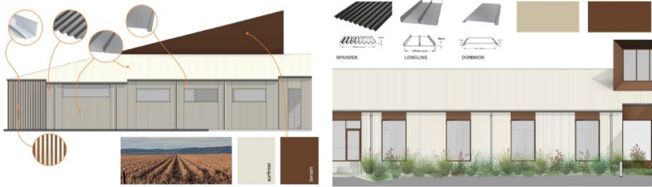
Figure 7 Façade Concept Typical Elevations
